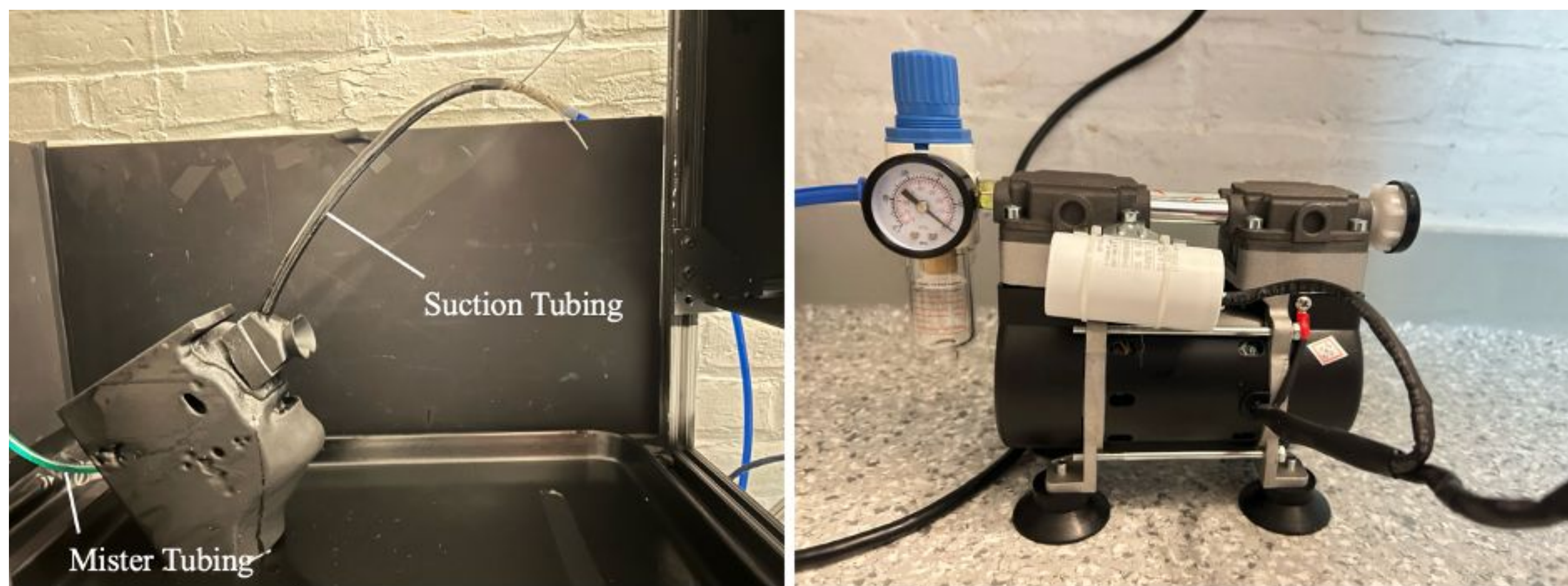
Figure 2. Experimental setup with the nasal port connected to controlled suction and a particle mister.
