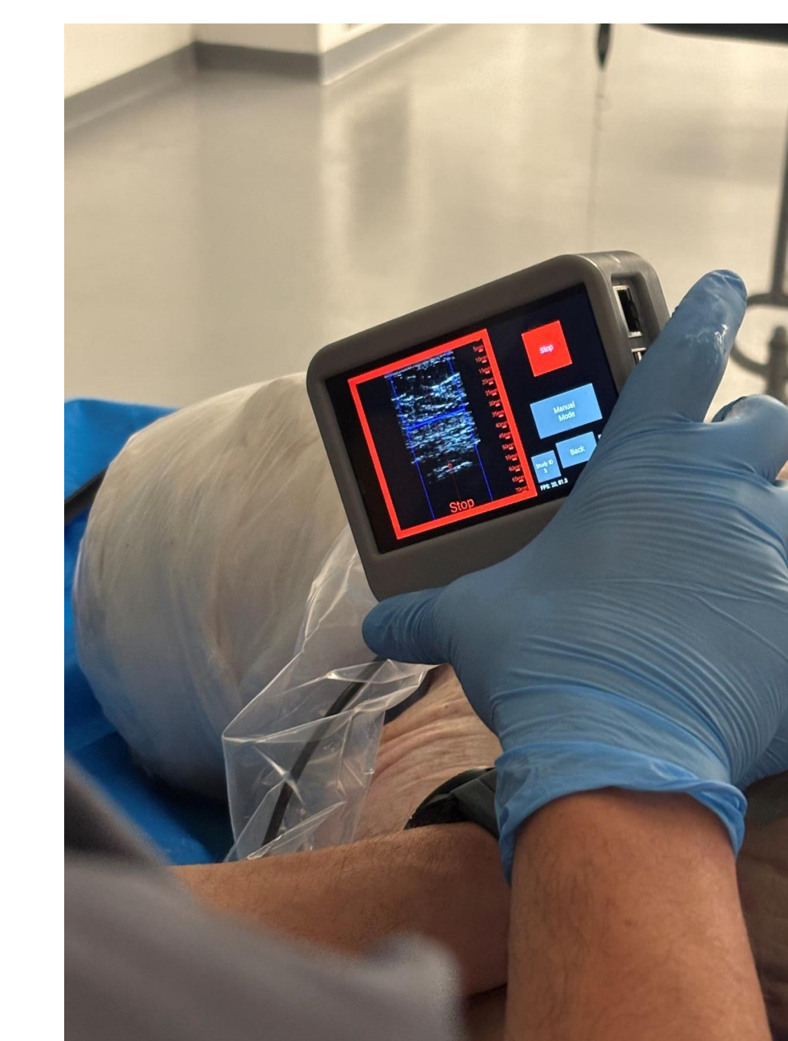
Image 2: The ANeED Device analyzing presence of pneumothorax during testing
